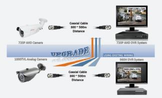
Multiple 1080p video streams can be easily transmitted using AHD over a single coaxial cable up to a length of 500 meters without any repeater. Unlike IP Cameras. AHD cameras transmit data that is not encoded resulting in no process and no delay real time and complete transmission.
